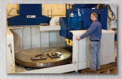
Tolerances of up to .002 flat and parallel can be held across the table depending on material, hardness and thickness.
