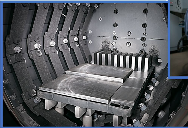
Kinetic's Abar Ipsen 6 bar 36" x 36" x 72" Vacuum Furnace
