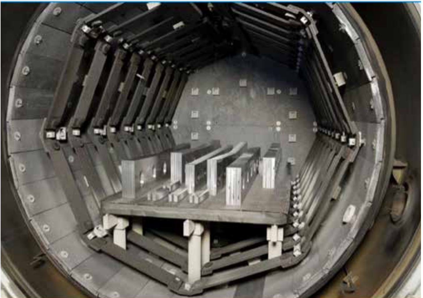
Figure 2. Inside a Vacuum Heat Treatment Furnace at Kinetic
