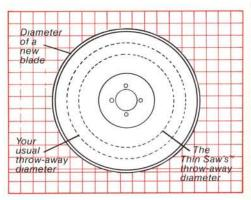
Extra blade life. You can grind The Thin Saw™ to a small diameter before you have to discard the blade The exact size of *your* throw away diameter depends on your mill practices
